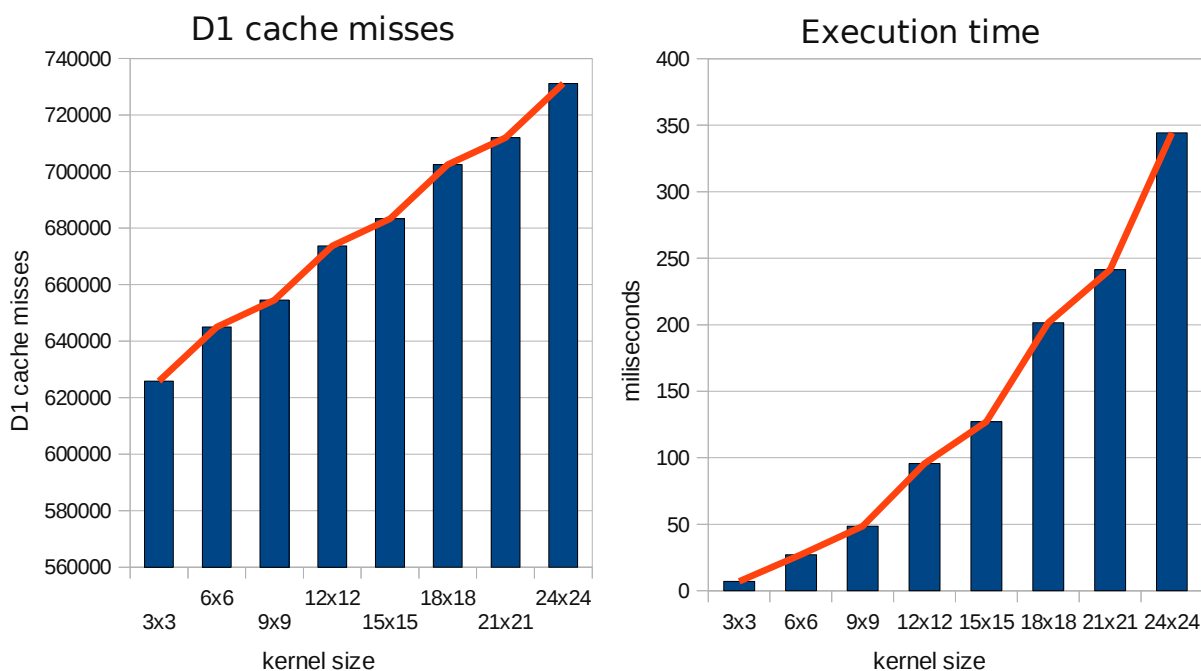
Figure 5 – D1 cache misses and execution time for different kernel sizes
